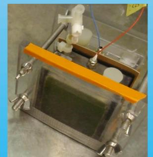
Photograph of a simple two-chamber bioelectrochemical system
