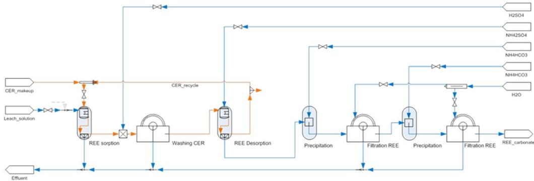
With sulfuric acid leaching and commercial cationites (macroporous M-31, Dowex) as sorbents extraction efficiency of 60-65 % has been gained. Derivatives were prepared as  $\text{Ce}_2\text{O}_3$  and as light REE and heavy REE carbonate based concentrates of 99,3-99,7% purity. A multicomponent process model has been developed at VTT (Co-op agreement RFMEFI58114X0002).
