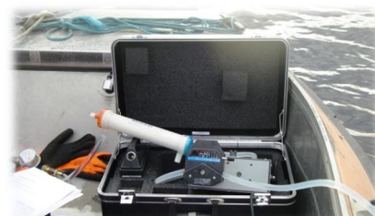
Concentrating water sample into sterile cartridge in Lake Kiantajärvi.
