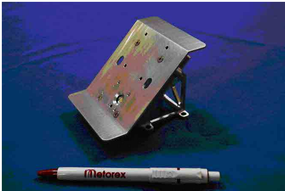
Figure 14. SMART-1 X-ray Solar Monitor sensor with the front-end electronics. The total size of the system is of the order of a mobile phone.
