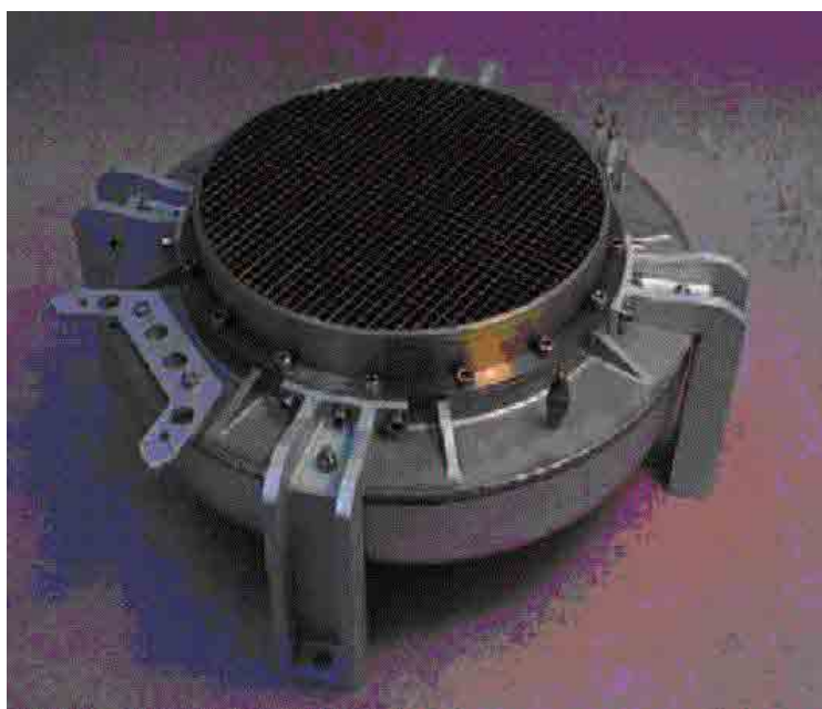
Figure 13. The JEM-X X-ray monitor sensor package for the INTEGRAL mission. The diameter of the collimator grid is close to 30 cm.
