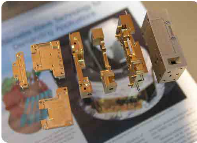
Figure 3. Low Frequency Instrument LFI 70 GHz Front-End Module. This compact matchbox size component houses four MMIC low noise amplifiers and two-phase shifters.
